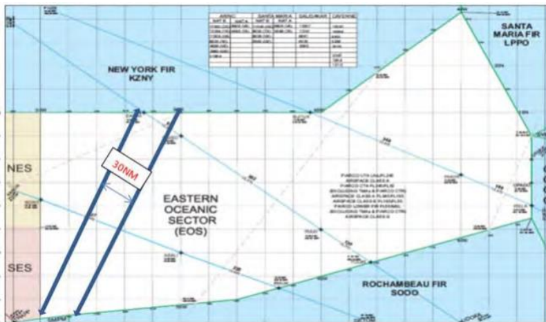
RNP 4 WILL ENABLE A REDUCTION FROM 50NM TO 30NM LATERAL SEPARATION and 30NM LONGITUDINAL SEPARATION MINIMA
